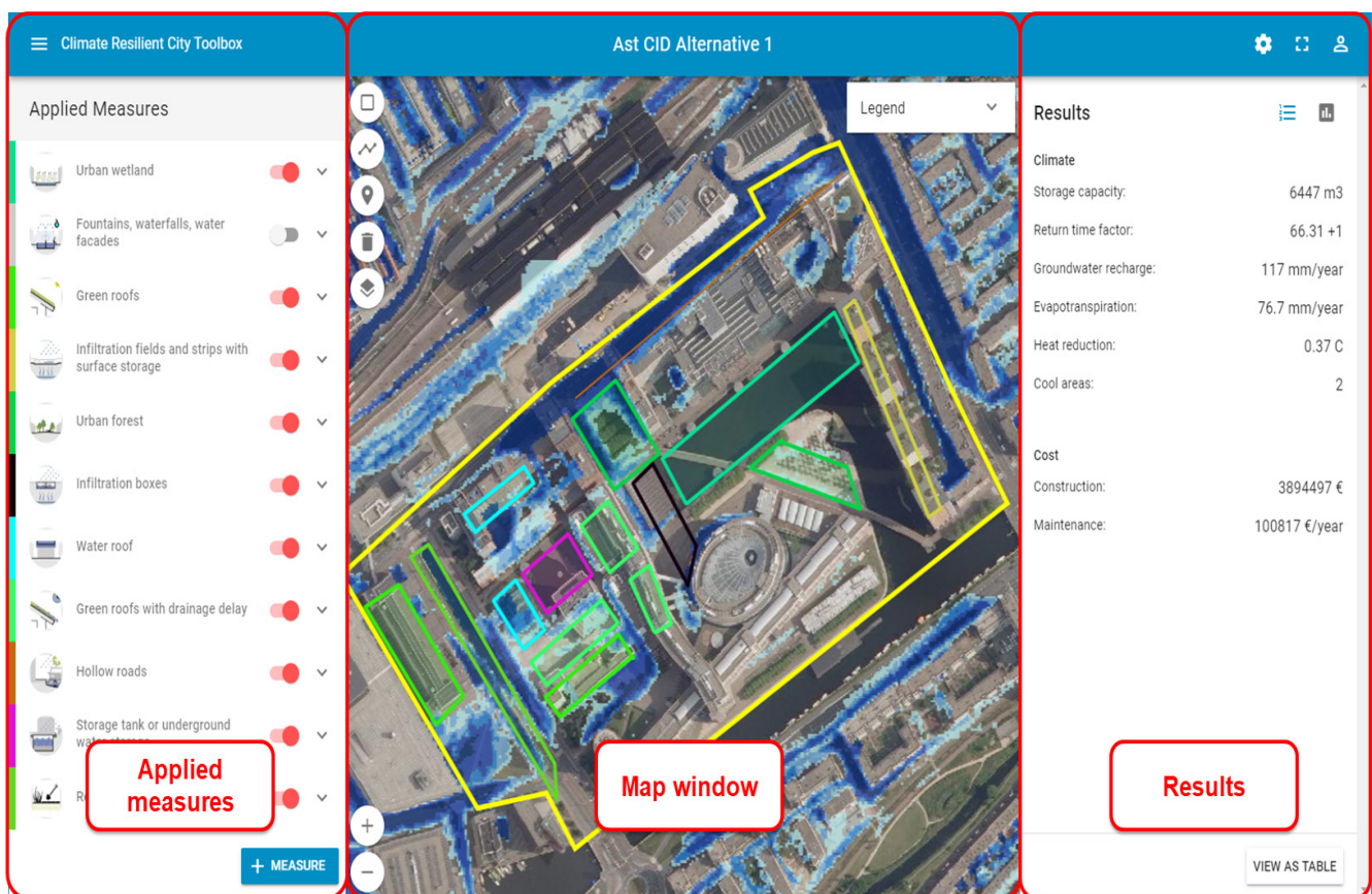
Image 3 : This picture displayed a screenshot of the CRC tool. This picture displayed a screenshot of the CRC tool. The window on the left shows the adaptation measures that have been chosen. A map of the project area is in the middle. The left window summarised the results of the measures describing its effects (e.g. on groundwater recharge, water quality, heat reduction) and providing an estimate of the costs for construction and maintenance. Source: Deltares
